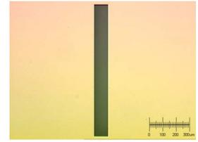
Figure 4 Etched line positioned at the center of the reference film.
